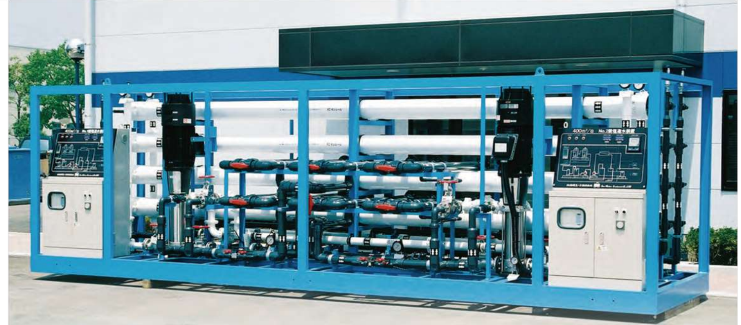
Brackish water desalination plant
